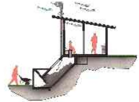
A compost toilet is one of the simplest and most effective methods to save water and to use the valuable biomass we produce to make the land more fertile instead of flushing it away as is done in a water closet.
