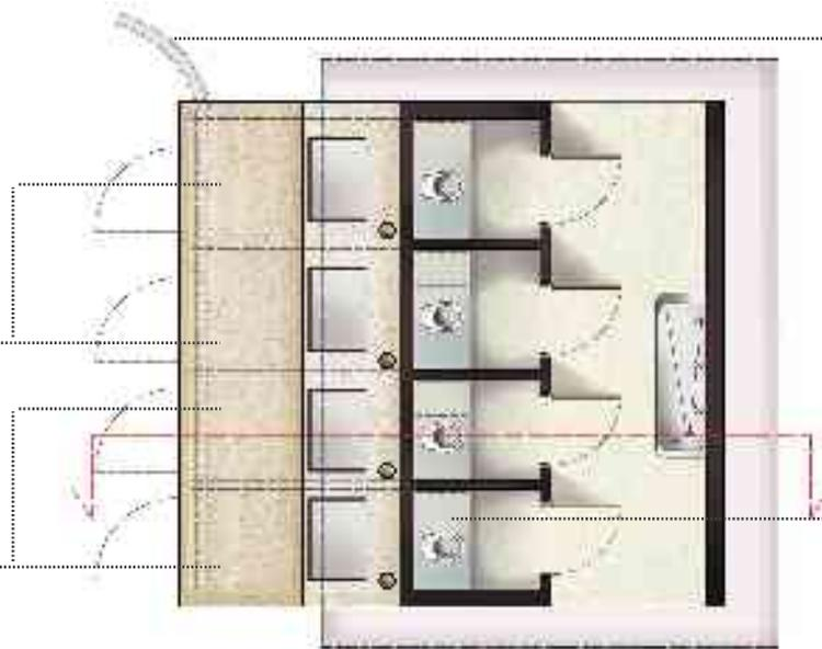
Drainage pipe to carry fluid to waste water treatment system. Urine and other liquids leave the compost toilet through a 10 - 16 cm diameter drainage tube near the lowest point in the system. These liquids then enter the plant-based water treatment system.
